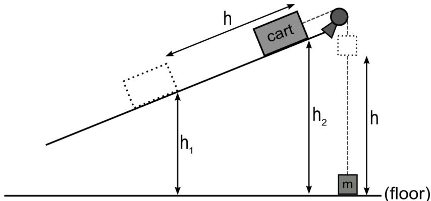
Before the cart and hanging mass are released (“initial” positions), we can write down the two objects' potential energies. There will be no kinetic energy, because there is no movement.
